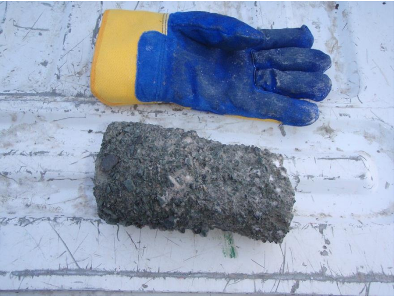
Photo 3: Drill core HB12-ND-CORE-DC24-QA-20120206. Coring stopped after grinding noises were heard.
