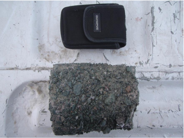
Photo 4: Drill core HB12-ND-CORE-DC25-QA-20120206. Poor quality due to lost circulation and loosened gravel.
